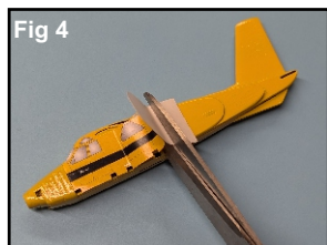
Fig 4 Slowly remove the backing by cutting in stages to make sure the decal is staying aligned on the surface.
