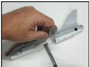
Slowly remove the backing by cutting in stages to make sure the decal is staying aligned on the surface.
